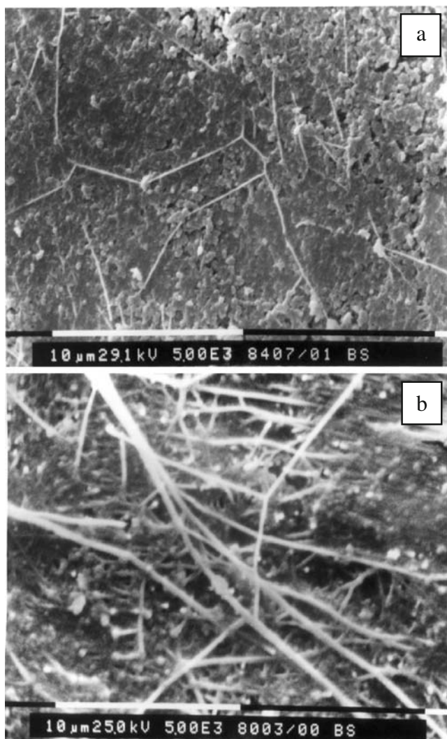
Fig. 2 SEM micrographs of a GDM and b fresh Co–Ni–Te–O film with R_{\text{Ni/Co}}=0.4 deposited on GDM
